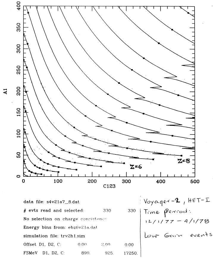
Fig.33 Fit of simulation tracks to A-stopping experimental events (Voyager-2, HET-I) registered in the time period of 12/1/77 to 4/1/78. The events are represented by energies deposited in A1 and C123 detector layers.
