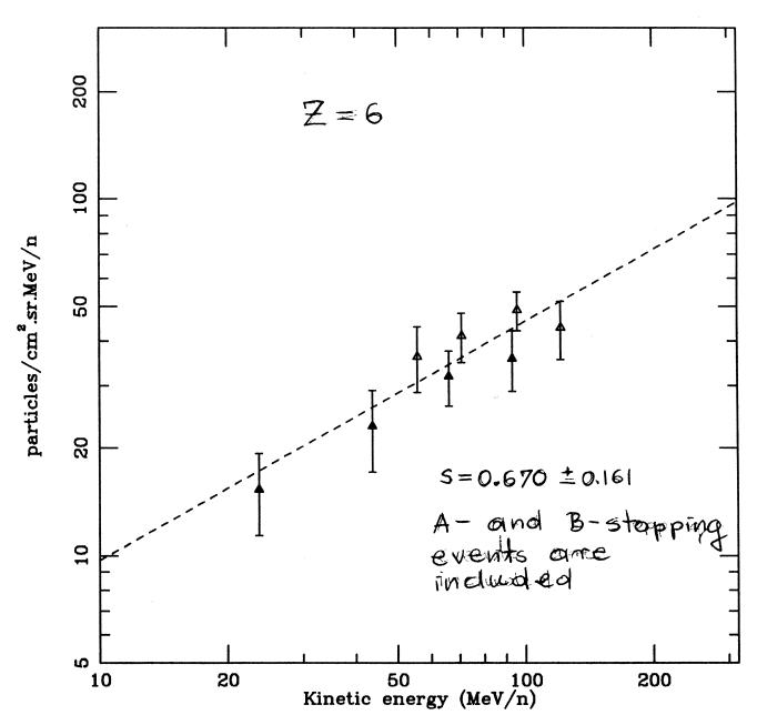
C:  $\triangle$  AS flv11a7\_8.dat  $\triangle$  BS flv11b7\_8.dat Fitted Galactic spectrum:  $dJ/dE = 0.691E-01*E^{0.670+-0.161}$  All fluxes times 30.0 TimeAS/TimeBS = 1.000
