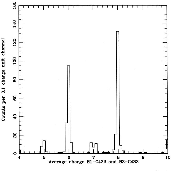
Fig.20 Number of counts versus charge Z for B-stopping events registered by Voyager-1 detector HET-II in the time period of 12/1/77 to 4/1/78.
