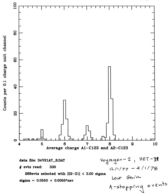
Fig.21 Number of counts versus charge Z for A-stopping events registered by Voyager-2 detector HET-I in the time period of 12/1/77 to 4/1/78.
