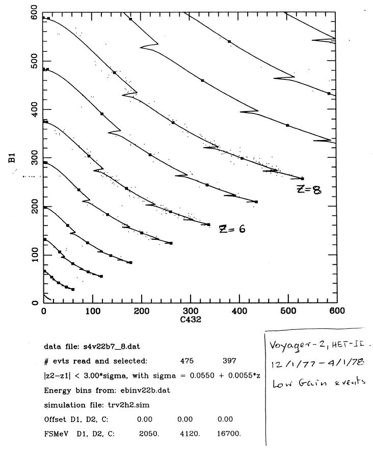
Fig.39 The same as in Fig.37 for the energies deposited in B1 and C432 detector layers.
