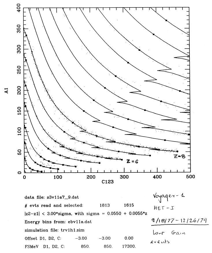
Fig.1 Fit of simulation tracks to A-stopping experimental events (Voyager-1, HET-I) registered in the time period of 9/18/77 to 12/26/79. The events are represented by energies deposited in A1 and C123 detector layers.
