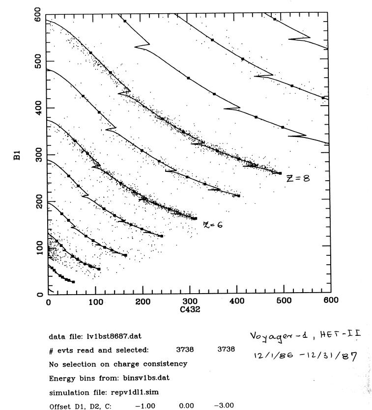
Fig.7 The same as in Fig.5 for the energies deposited in B1 and C432 detector layers.
