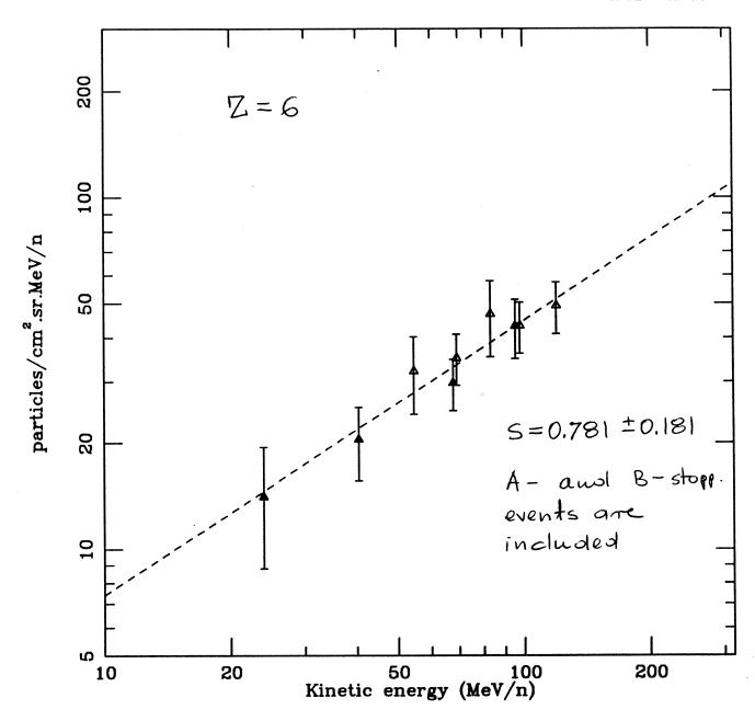
C:  $\triangle$  AS flv1asbin5.dat  $\triangle$  BS flv1bsbin5.dat Fitted Galactic spectrum: dJ/dE= 0.408E-01\*E  $^{0.781+-}$  0.181 All fluxes times 30.0 TimeAS/TimeBS = 1.000
