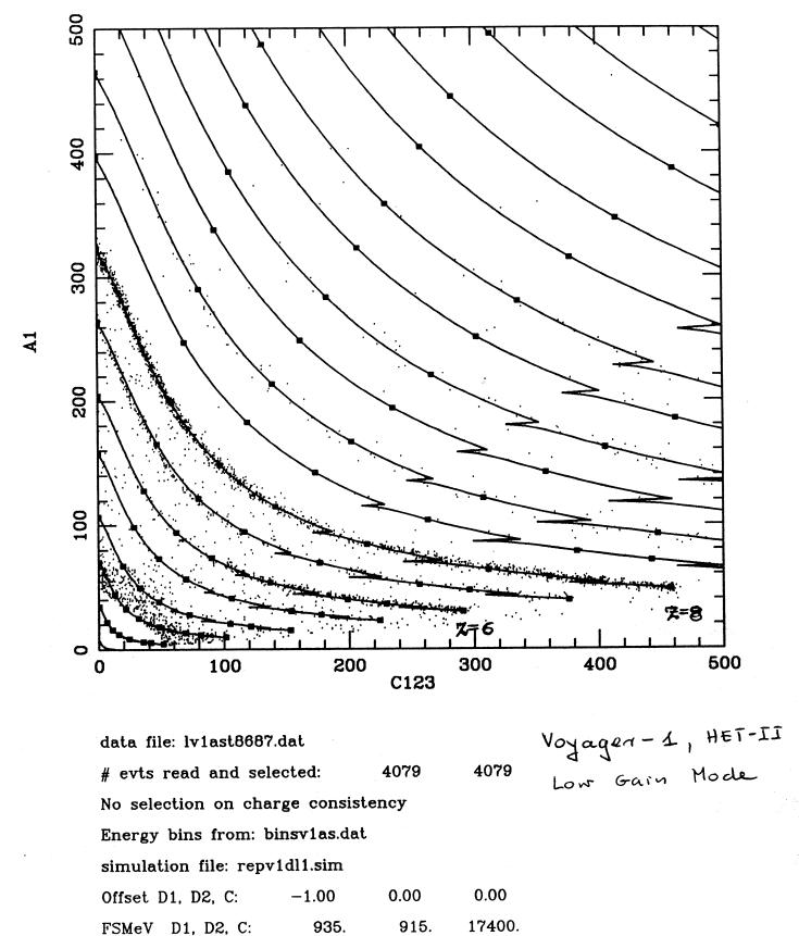
Fig.5 Fit of simulation tracks to A-stopping experimental events (Voyager-1, HET-II) registered in the time period of 11/1/86 to 12/31/87. The events are represented by energies deposited in A1 and C123 detector layers.
