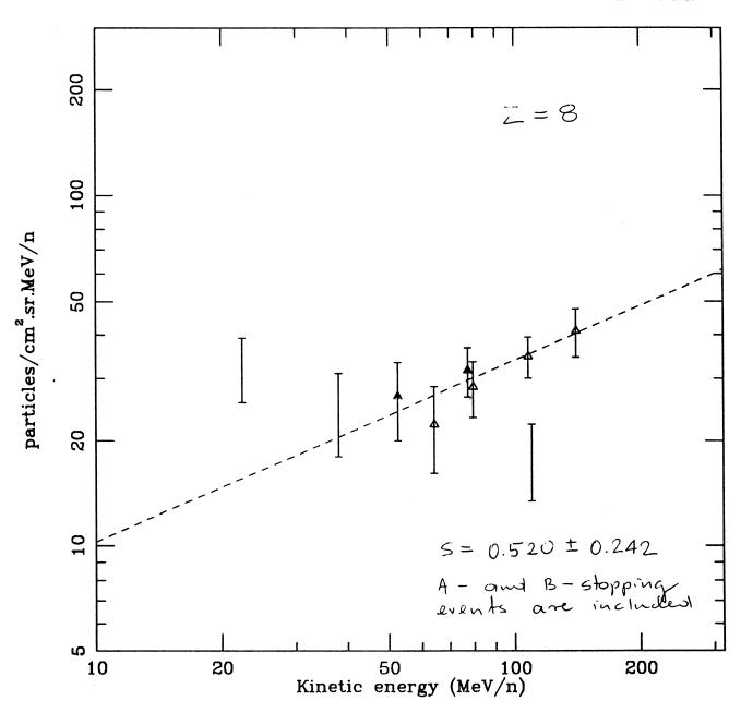
0:  $\triangle$  AS f8v21a7\_8.dat  $\triangle$  BS f8v21b7\_8.dat Fitted Galactic spectrum:  $dJ/dE = 0.103E + 00*E^{-0.520+-0.242}$  All fluxes times 30.0 TimeAS/TimeBS = 1.000
